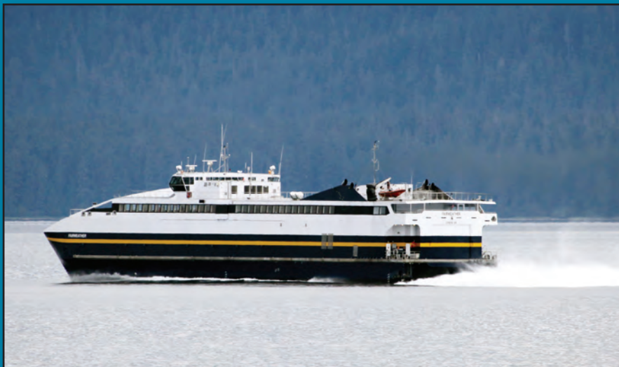
The Alaska Marine Highway's M/V Fairweather cruises through Stephen's Passage on its summer run to Petersburg. Delivered in 2004, the 235 ft vessel operates at 32 knots with a maximum speed of 43 knots.
